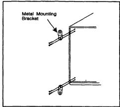
5. Install four screws in the wall studs according to the dimensions given in Figure 3-3. (Note that the width dimension is different for the DBS 40.)
