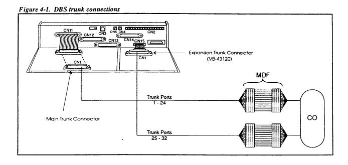
The number of trunks that can be connected through the main trunk connector depends on the type of system you have and the number of trunk cards installed. Table 4-1 shows the main trunks and expansion trunks available with each system type. Chapter 6 includes trunk maximums for two-cabinet systems.
