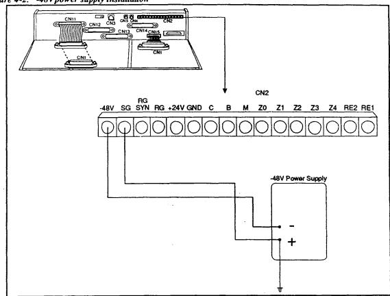
3. Ground the positive side of the -48V power supply to the building ground.
