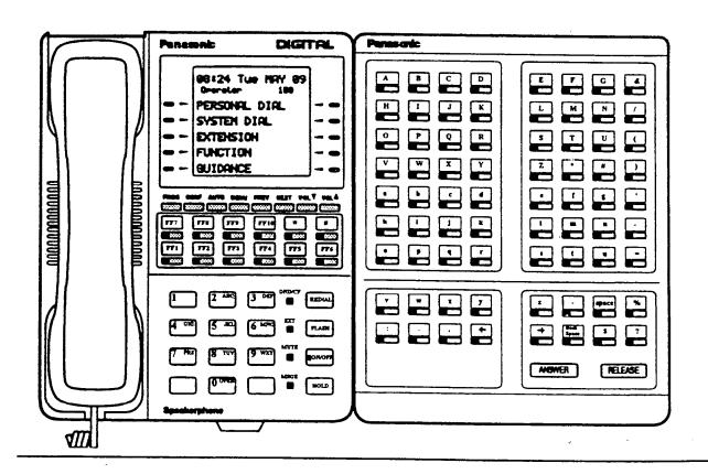
When the Attendant Feature Package (VB-43330) is installed, the DSS/72 can be used as an Attendant Console. The attendant console provides station monitoring and call transfer by name for large systems, even if a large display phone is not used.
