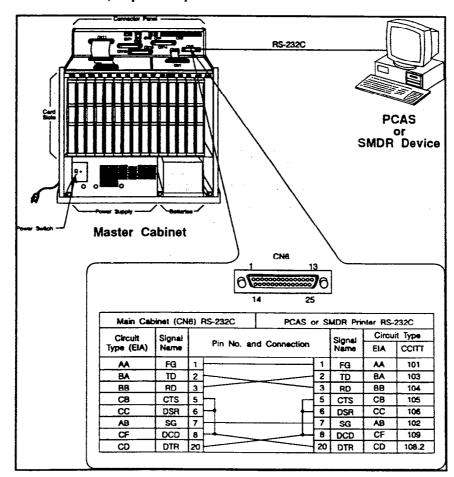
Figure 5-1. RS-232C connection, 25-pin to 25-pin
